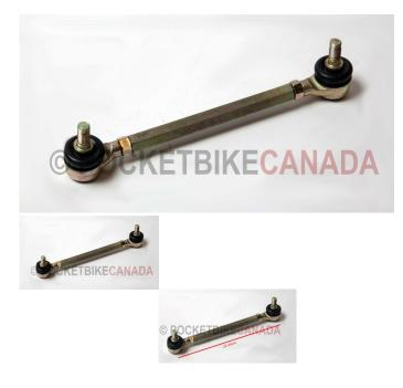
Steering Tie Rods w/ Ball Joints for 110cc, YL110/Mini Viper, ATV Quad 4-Stroke - G1030035
